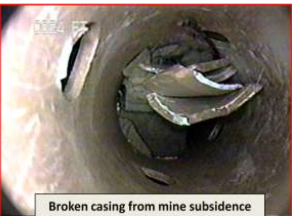
Cracked casing seen by side-viewing mirror
